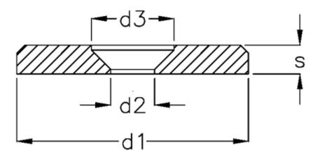
$\begin{array}{ll} \text{Countersunk screw} = \text{M6} \\ \text{d1} & = 52 \\ \text{d2} & = 6.4 \\ \text{d3} & = 12 \\ \text{s} & = 6.0 \\ \end{array}$
